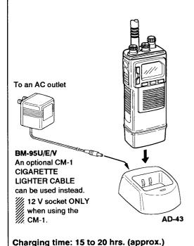
♦ When charging in unstable places such as aboard a ship, use the supplied self-tapping screws, or nuts and bolts, plus the inserts to stabilize the AD-43 to a solid, flat surface and prevent the transceiver from popping out of the AD-43.
