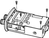
② Remove the 4 P. C. board screws.
