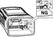
**CAUTION:** Make sure the 2 bottom screws are securely tightened to ensure that the transceiver remains wateright and no water is able to seep inside the casing.
