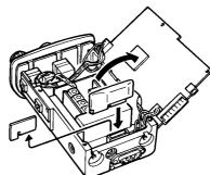
③ Open the P. C. board; then, remove the small unit and install the scrambler unit in itsplace.
