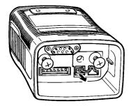
(1) Unplug the connector, loosen the 2 bottom screws; then remove the case.
